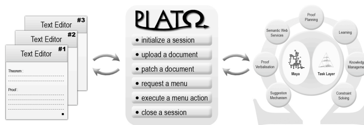
Figure 1: Architecture of the integration of \text{\TeX}_{\text{MACS}} and the \Omega\text{MEGA} system via PLATΩ
